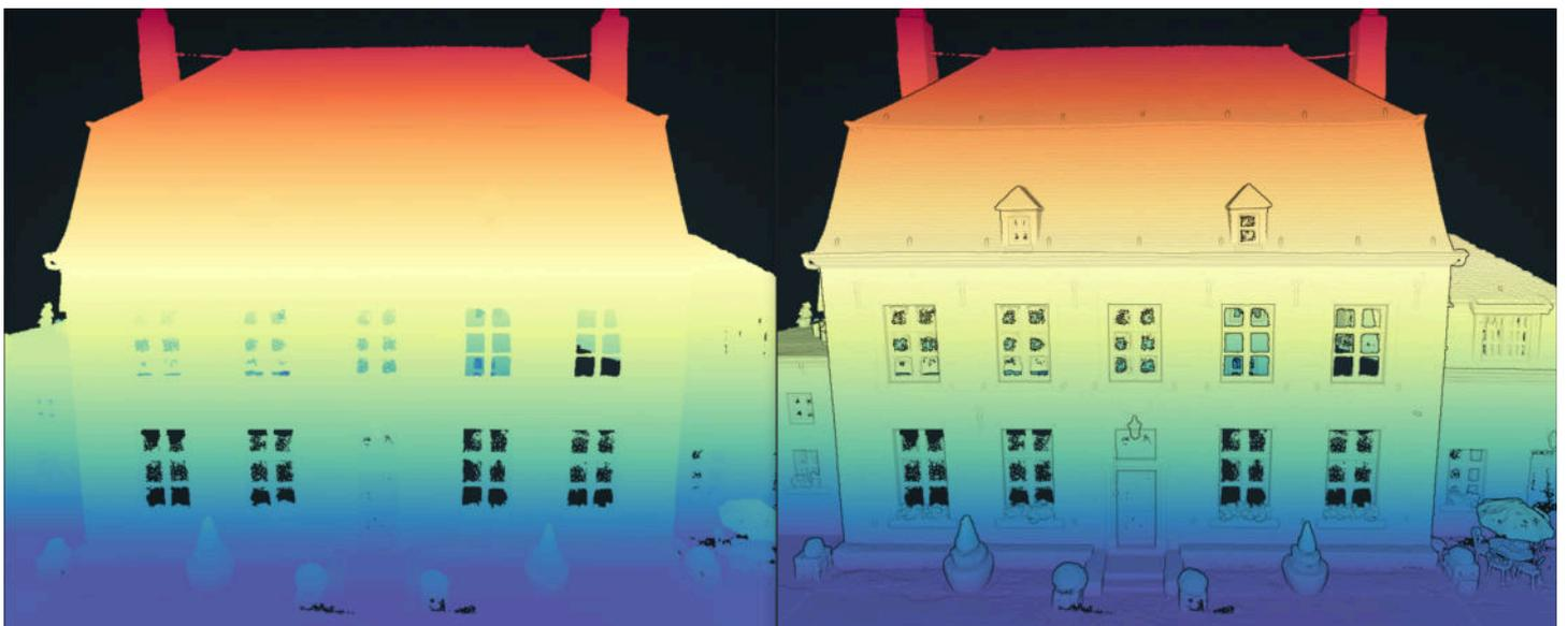
Same point cloud without EDL (left) and with it (right), Radius and Strength parameters impact the degree of edge shadowing @ULB
